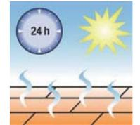
Allow to dry. Do not wet or dirty the surface for 24 hours
