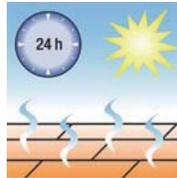
Allow to dry. Do not wet or dirty the surface for 24 hours
